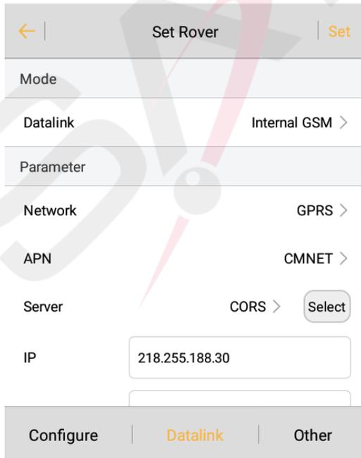
Figure 3-3-3 Internal GSM
