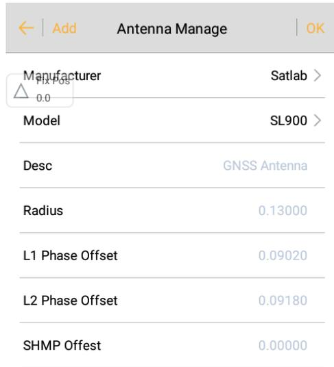
Figure 3-1-10 Antenna Manage
