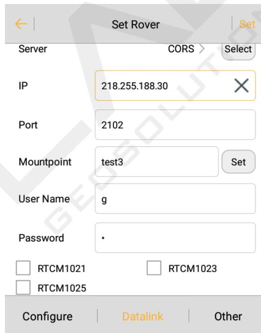
Figure 3-3-7 CORS Parameters
