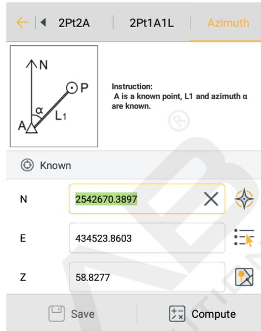
Figure 6-6-6 Azimuth Interface
